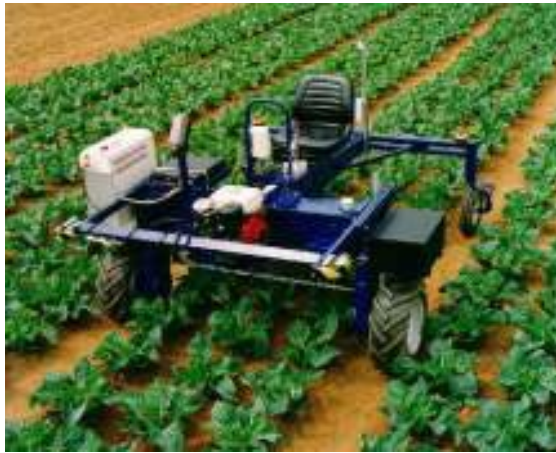
Figure 23. The tool frame tractor used as a platform for the 2008 trial.
