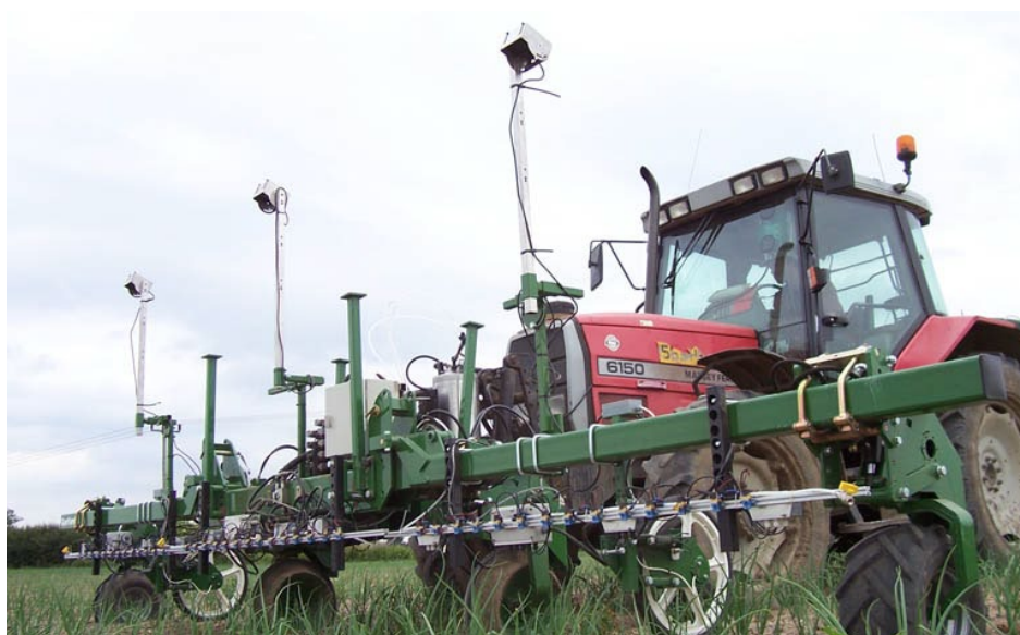
Figure 29. Three section experimental spot sprayer based on a Garford cultivator tool frame.
