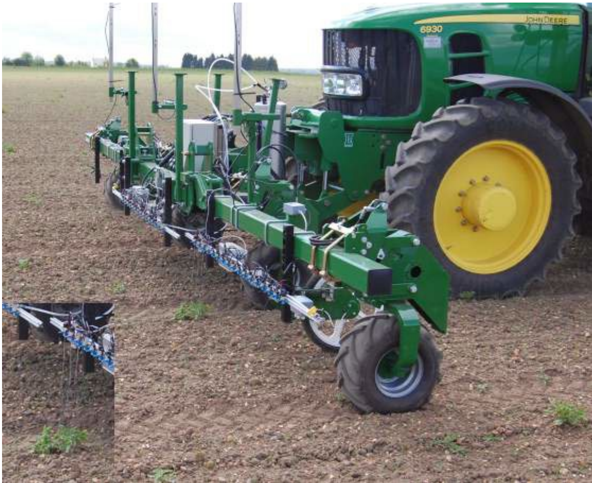
Figure A. Full-scale field rig operating in an onion crop (Inset showing nozzle operation).
