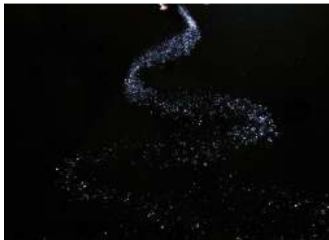
Figure 10. Spray formation from a fluidic nozzle with an oscillating jet.
