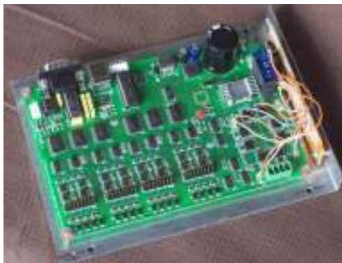
Figure 25. The microcontroller sprayer board - custom designed and built for this project.
