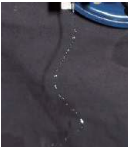
Figure 13. View of droplets forming out of a jet issuing from a mechanically oscillating tube.
